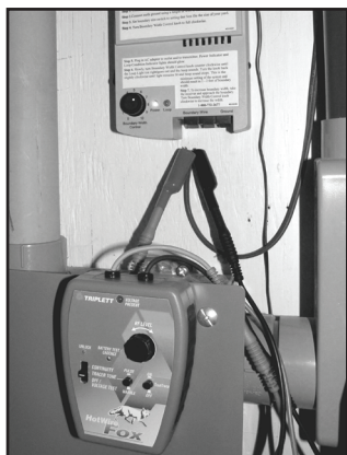
HotWire Fox connected to boundary wires
