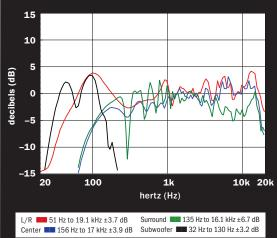
The C336 tower's measurements indicate a wide floor bounce centered at 200 Hz, followed by narrow band irregularities beginning at 800 Hz. The CC225 center displays a similar character at higher frequencies, along with low-frequency response that falls quickly below 400 Hz. Overall,
