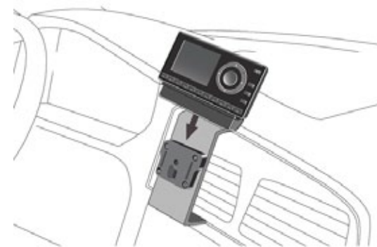
Mounting the Plug and Play Unit with a 'Pro Clip' accessory available on Amazon.com
