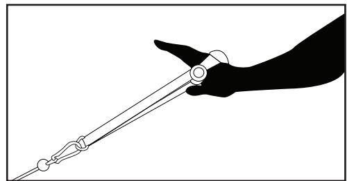
**Ankle Cuff Grip:** The cuff opening can be made larger to accommodate the ankle. Place your hand in the cuff and slide it away from the grip. Insert your foot or ankle and tighten by sliding the grip back toward the cuff.
